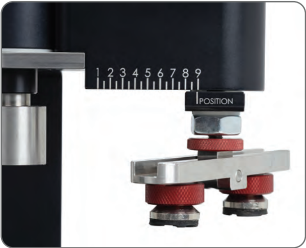
Graduations enable quick, repeatable pad positioning when using different size sample holders.
