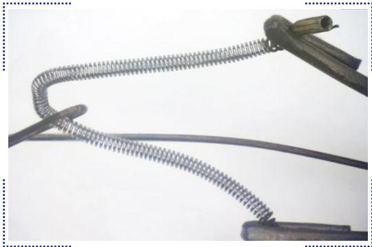
Light Bulb Filament inspected by ZEISS Visioner 1
